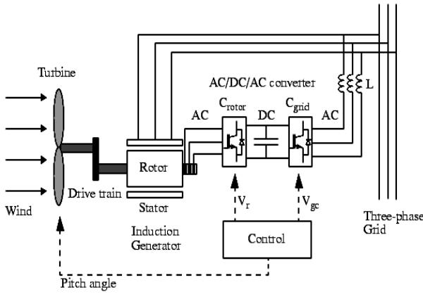
Fig. 2. The Wind Turbine and the DFIG System
