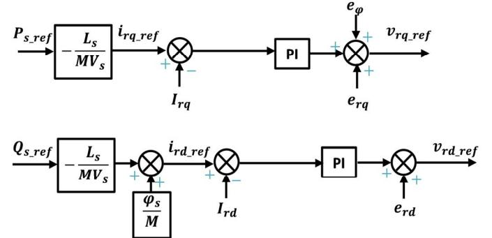
Fig. 4. Model of the field oriented control of DFIG
