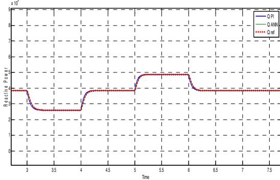
Fig. 11. Reactive power of wind turbine injected after disturbances
