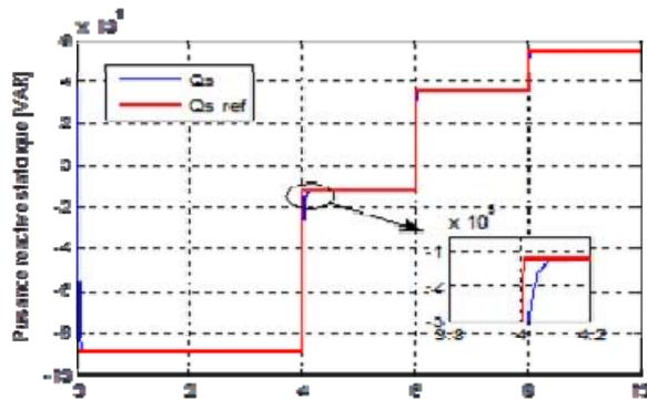
Fig. 5. Reactive power of DFIG using F.O.C
