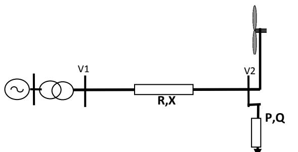
Fig. 7. A Single machine power system with wind generator
