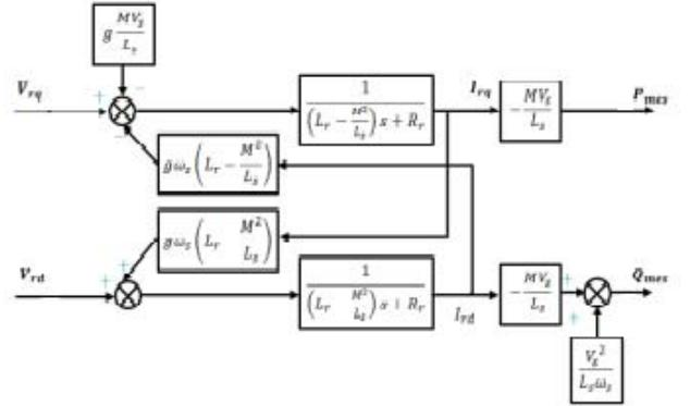
Fig. 3 Simplified Model of the DFIG
