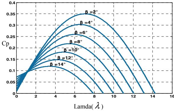
Fig 1: Power coefficient based on the ratio of speed
