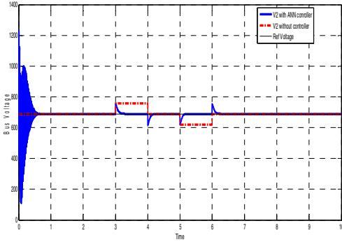
Fig. 12. Voltage control using reactive wind controller
