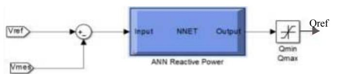
Fig. 9. ANN controller Simulink model for reactive power.
