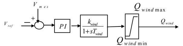
Fig. 8. Reactive wind power controller.
